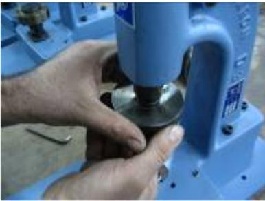
3. put in the lower die to the lower die slot and screw its hexnut by the key as shown at the photos below
