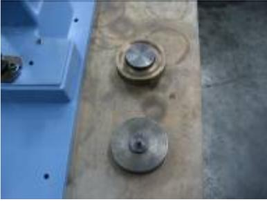
2. screw the upper die tightly the direction of anticlockwise as shown at the photo below
